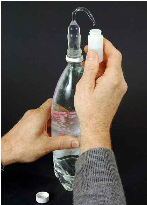
Figure 1 Extracting the oil/scintillant from the PET bottle after slowly shaking the water/oil mixture.
