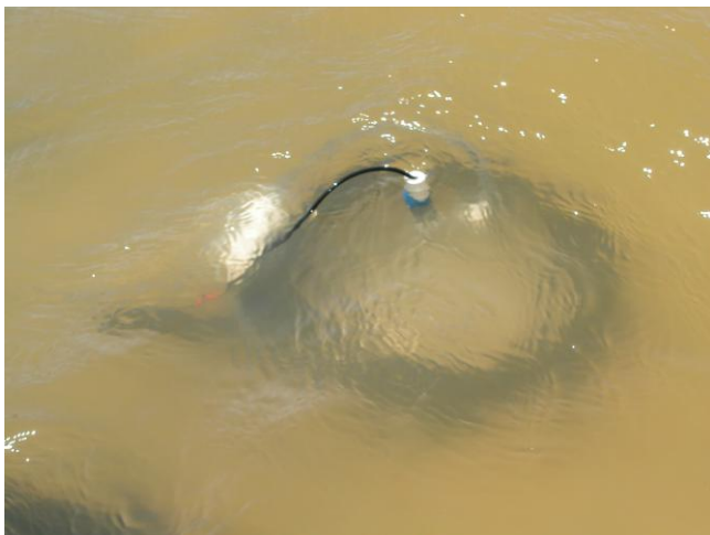
Close up of a light chamber showing the DO sensor and the inline submersible pump to circulate water within the chamber
