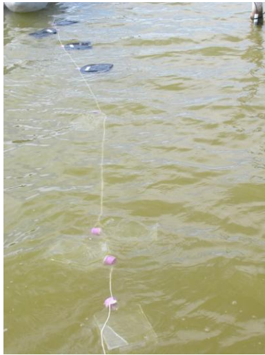
Dark and light bottles being incubated in situ for phytoplankton productivity measurements
