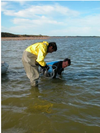
Deployment of chambers on the sediments for phytobenthic productivity measurements
