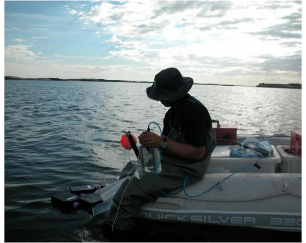
Measuring changes in dissolved oxygen prior to and after incubation to assess phytoplankton productivity
