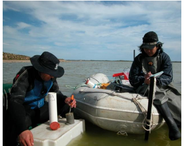
Sampling phytobenthic biomass from sediment cores
