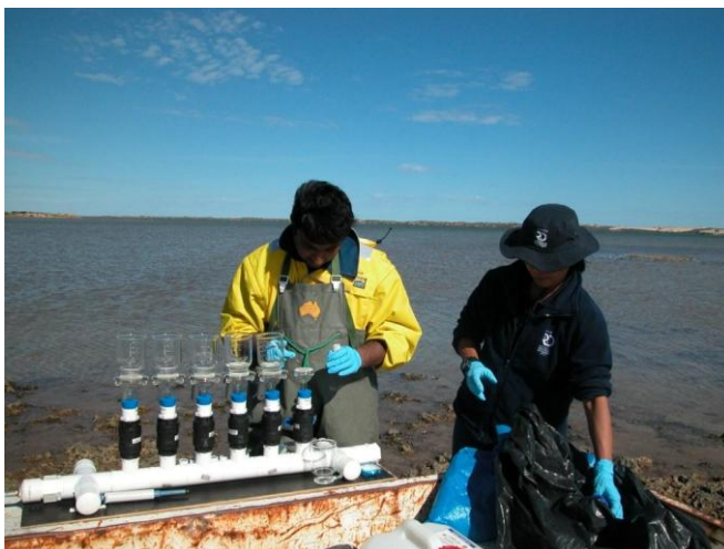
Dark and light bottles being incubated in situ for phytoplankton productivity measurements
