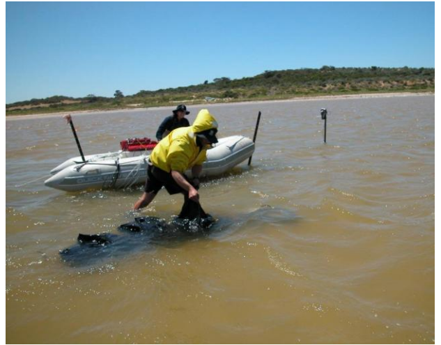
Placing weighted dark plastic bags to simulate dark conditions
