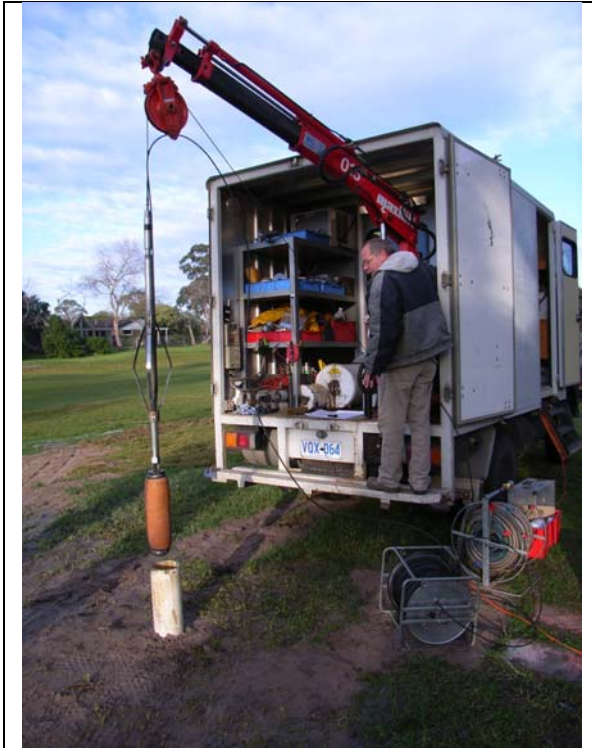
EMF testing of BH4. Don Freebairn (DWLBC) is shown lowering the flowmeter and packer assembly down the well. Two reels containing the pressure delivery tubing and monitoring pump can be seen on the bottom RHS of the image.
