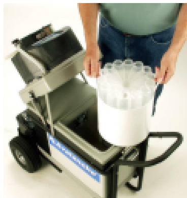
Figure 14. ISCO Avalanche refrigerated auto-sampler and bottle carousel (Source - Avensys)
