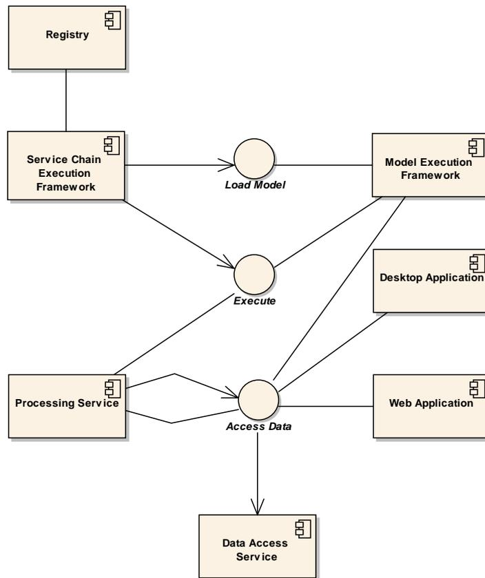
**Figure 4-9: Examples of Interfaces Between WRON Resources and Resource Users**
