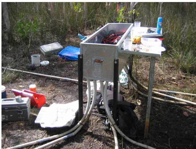
Figure 12. Heat pulse system showing locking storage box mounted on posts and conduits carrying cables entering through the underside of the box.
