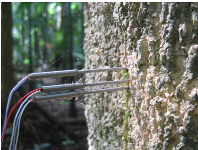
Figure 14. Installed heater and thermistor probes.
