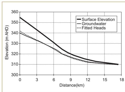
**Figure 14.** Measured and fitted steady state groundwater heads in the Gunnedah Formation for Yarramanbah Creek catchment. The RMSE between the observed and calculated heads is 0.70 m.
