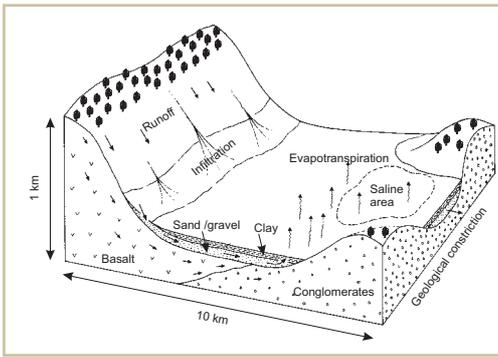
**Figure 3.** Block diagram presenting the conceptual model for the hydrogeological processes on the salt affected catchments on the Liverpool Plains: recharge occurs at the break of slope and due to the bedrock highs at the outlet of the groundwater catchment, discharge to the surface occurs resulting in a saline area.
