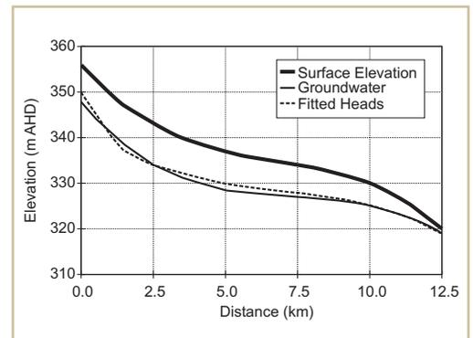
**Figure 15.** Measured and fitted steady state groundwater heads in the Gunnedah Formation for Pump Station Creek catchment. The RMSE between the observed and calculated heads is 0.85 m.
