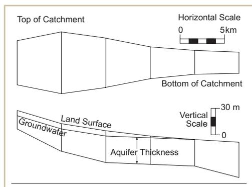
Figure 7. Plan view and cross section of Big Jacks Creek catchment, as discretised from available bore lithology information presented in Dyce and Richardson (1997). Note that aquifer thickness does not indicate the depth below surface of the aquifer, only the average thickness of material.
