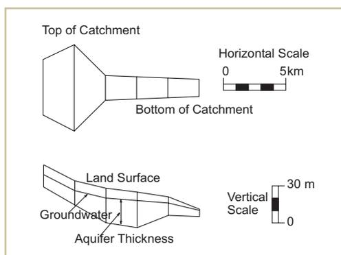
Figure 9. Plan view and cross section of Pump Station Creek catchment, as discretised from available bore lithology information presented in Dyce and Richardson (1997). Note that aquifer thickness does not indicate the depth below surface of the aquifer, only the average thickness of material.
