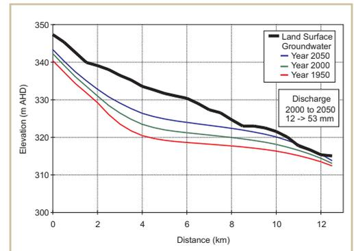
**Figure 19.** Transient water level simulation for estimated historical and future in the Pump Station Creek catchment
