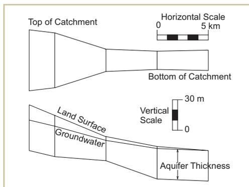
Figure 8. Plan view and cross section of Yarramanbah Creek catchment, as discretised from available bore lithology information presented in Dyce and Richardson (1997). Note that aquifer thickness does not indicate the depth below surface of the aquifer, only the average thickness of material.
