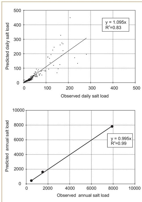
**Figures 25a and 25b.** Observed versus predicted (a) daily and (b) annual saltload from Big Jacks Creek, based on a modified power regression.
