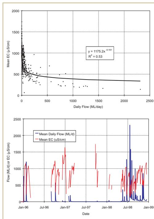
**Figures 23a and 23b.** Daily flow versus daily mean EC, and the time series of flow and EC for Big Jacks Creek, for the three year period 1996 to 1998.
