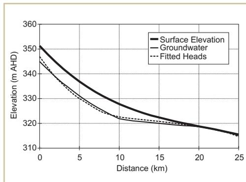
**Figure 13.** Measured and fitted steady state groundwater heads in the Gunnedah Formation for Big Jacks Creek catchment. The root mean square error (RMSE) between the observed and calculated heads is 0.69 m.
