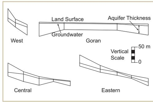
**Figure 11.** Cross sections for three arms and main trunk of the Lake Goran catchment, as discretised from bore lithology information presented in Dyce and Richardson (1997). Note that aquifer thickness does not indicate the depth below surface of the aquifer, only the average thickness of material.
