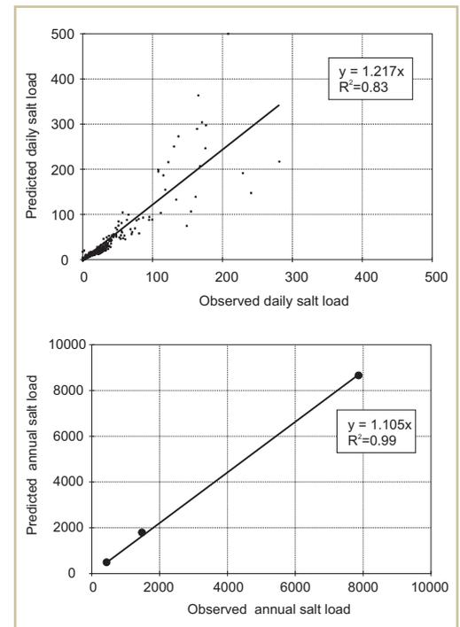
**Figures 24a and 24b.** Observed versus predicted (a) daily and (b) annual saltload from Big Jacks Creek, based on a simple power regression.
