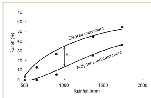
**Figure 5.** Relationship between rainfall and runoff adapted from Holmes and Sinclair (1986) (—); obtained from the WAVES model (•).
