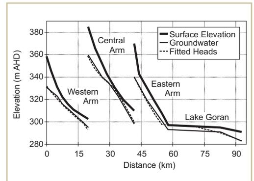
**Figure 16.** Measured and fitted steady state groundwater heads in the Gunnedah Formation for the Lake Goran catchment. The RMSE between the observed and calculated heads for each of the three arms and trunk varied between 1.17 and 2.71 m, and is 1.78 m overall.
