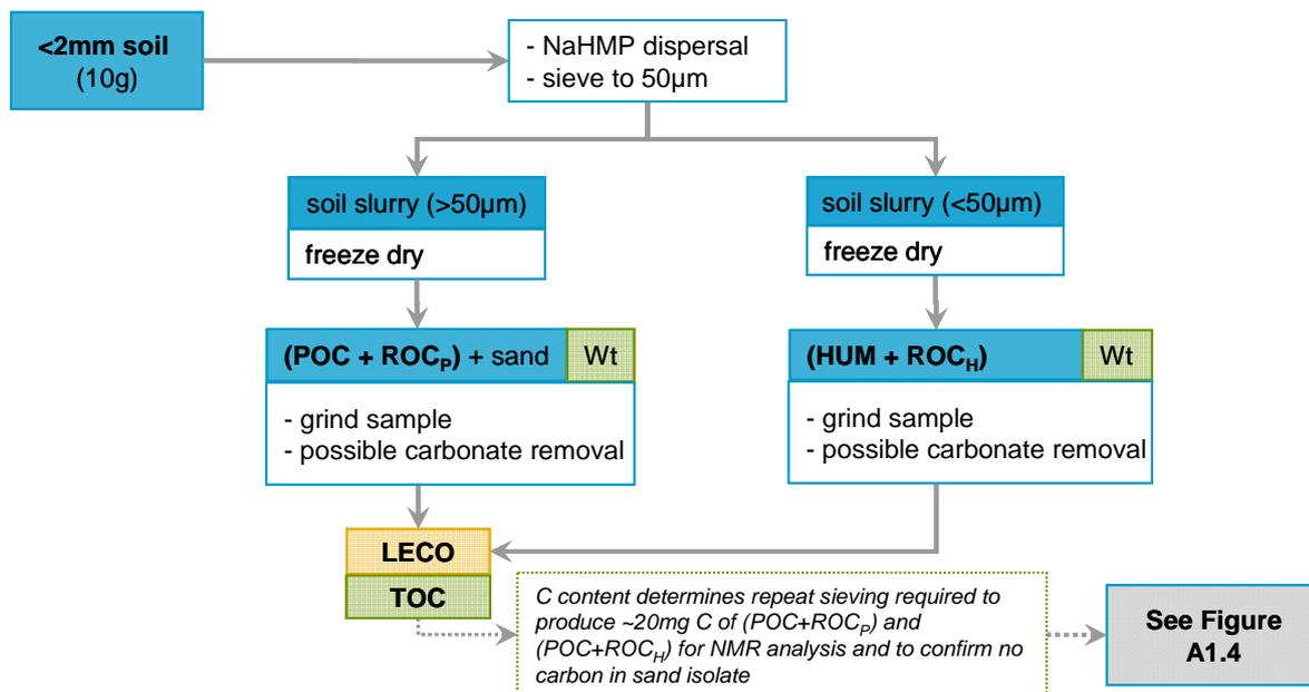
**Figure A1.4** Fractionation Part 2: Determination of Resistant OC
