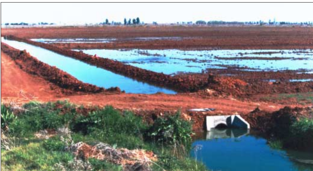
Sewage effluent being applied at the top of the FILTER plots during summer cropping
