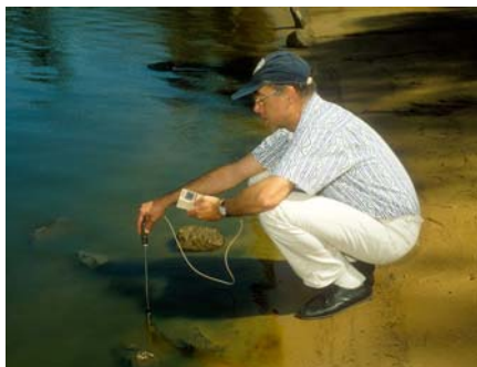
CSIRO scientist using a nephelometer to measure turbidity in water polluted by blue green algae
