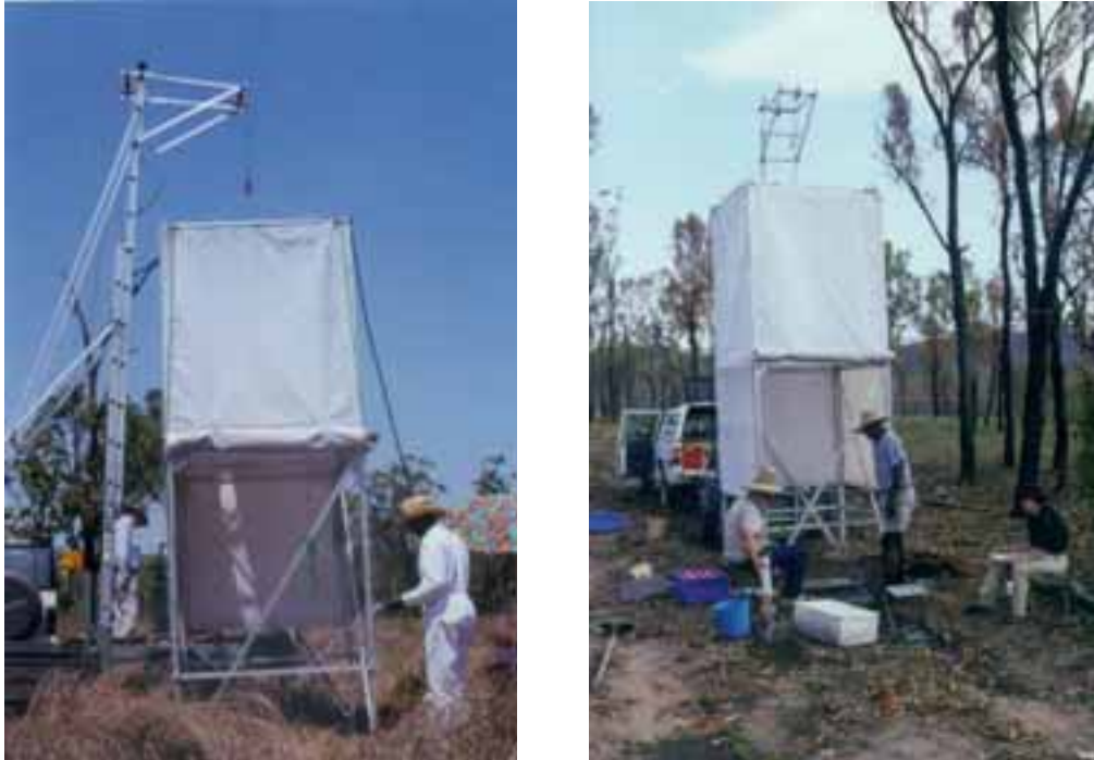
Figure 8.5: Views of the rainfall simulator in operation. Wind shield can be lowered in response to main direction of wind.
