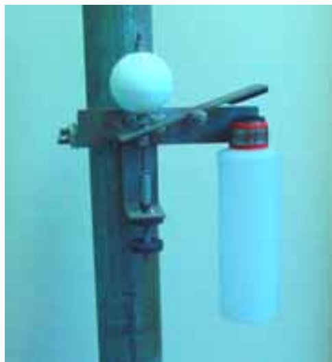
Figure 3.1: Single bottle sampler
