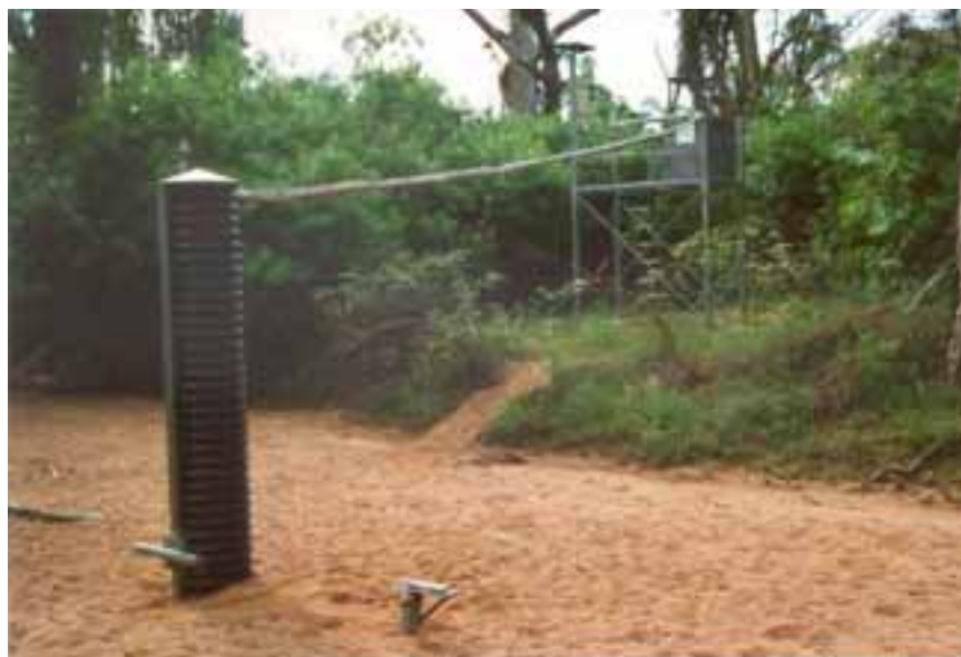
Figure 3.11: Gauging station at Wheel Creek. Sampling device with attached turbidity sensor and stand along flow velocity meter in foreground; platform with autosampler in background.
