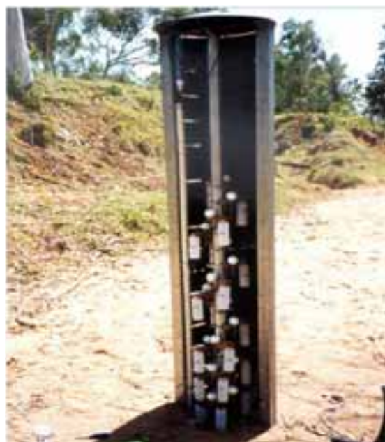
Figure 3.7: Arrangement of bottle samplers in enclosure at Weany Creek.
