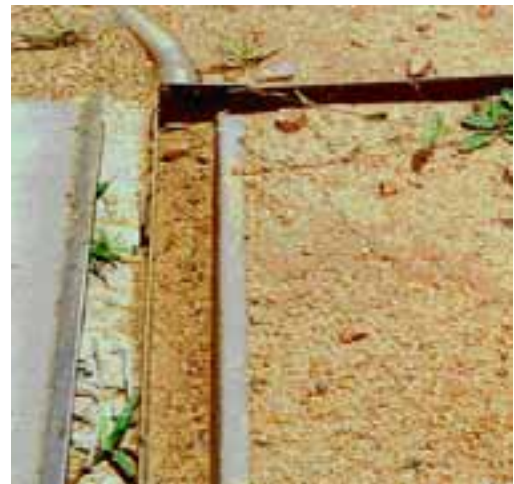
Figure 2.6: Coarse sediment trapped in trough
