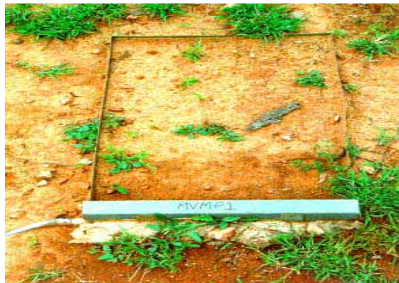
Figure 2.2: Microplot frame and trough
