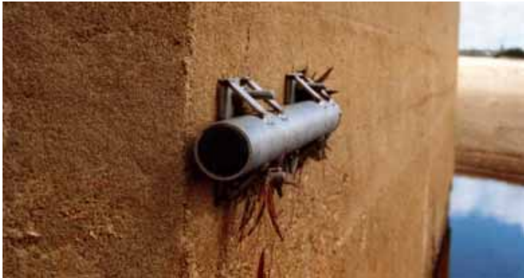
Figure 3.18: Turbidity meter inside the stainless steel housing, fixed to the old railway bridge at Macrossan on the Burdekin River.
