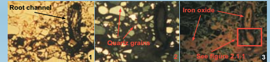
Figure 2.1. Thin section analysis of BG11, horizon 2Eg shows a pore (root channel) surrounded by orange Fe oxides. Field of view is 3.2 mm across. Image 1 is PPL, image 2 is XPL and image 3 is reflected light.
