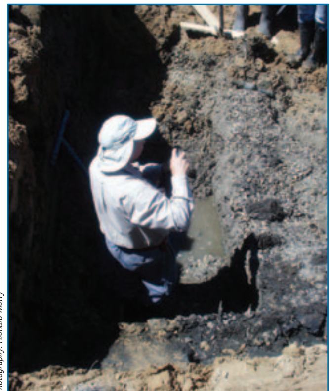
Figure 1b Potential acid sulfate soils showing dark sulfidic material ( \text{pH} 7 )
