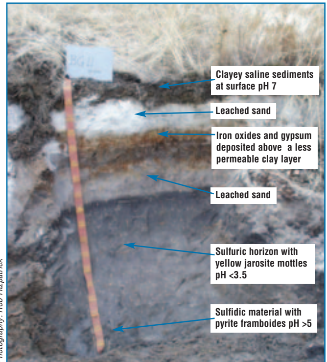
Figure 1a Actual acid sulfate soils showing yellow streaks and mottling patterns containing jarosite ( \text{pH} < 4 ) in the grey subsoil
