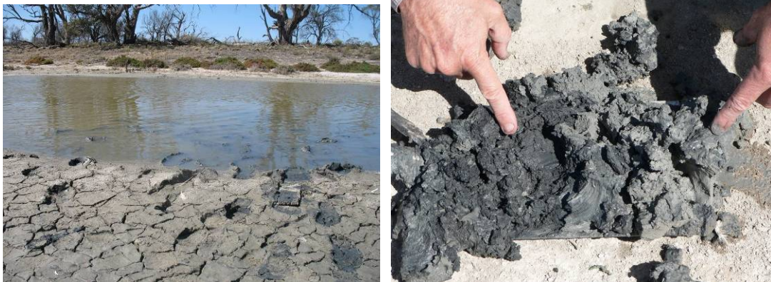
Figure 5 . Site TB5 sampled in water (subaqueous) near the sand-bagged outlet to the billabong (Left side). Sulfidic subaqueous clayey soil (wet, soft clayey sulfidic material overlying wet heavy clay sulfidic material) (Right side).
