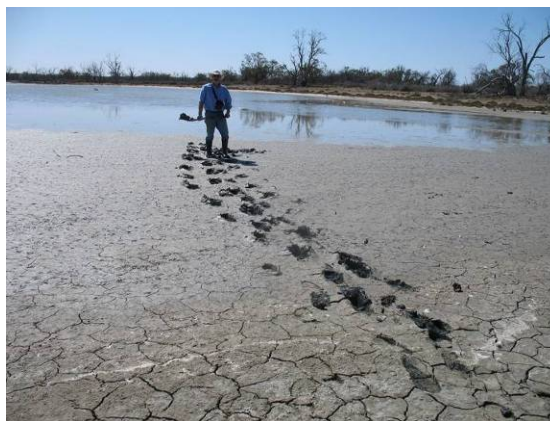
Figure 9. Sulfidic cracking clay soil near Site TB4 at the south-western end of Tareena Billabong. The top 5 cm has potential to acidify significantly, depending on drying.
