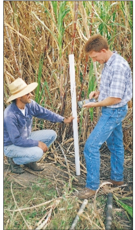
Installing a drainage meter in a Burdekin canefield
