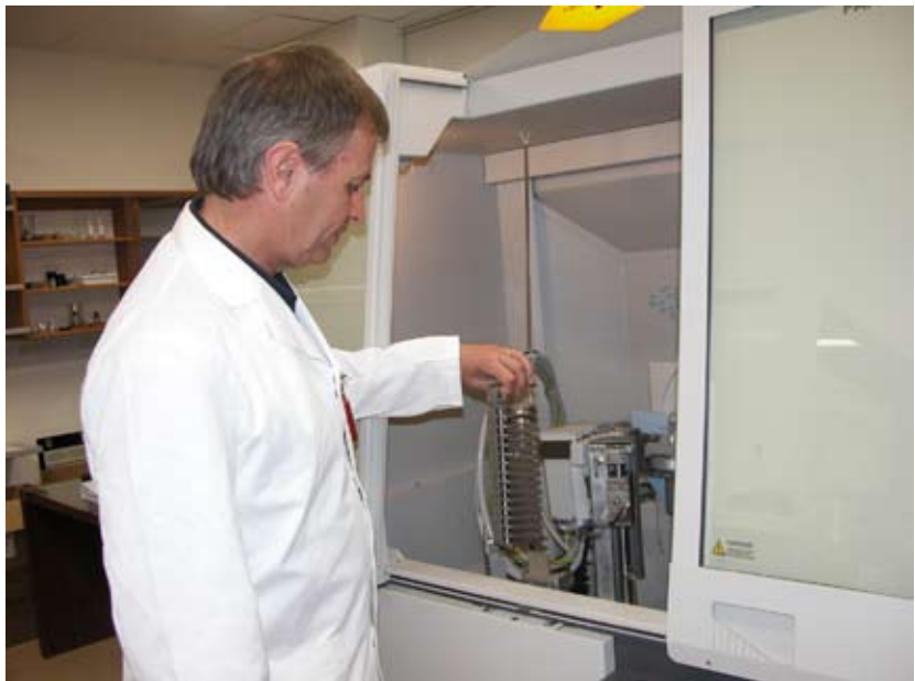
> CSIRO Land and Water researcher Mark Raven loading samples for mineralogical analysis using x-ray diffraction
